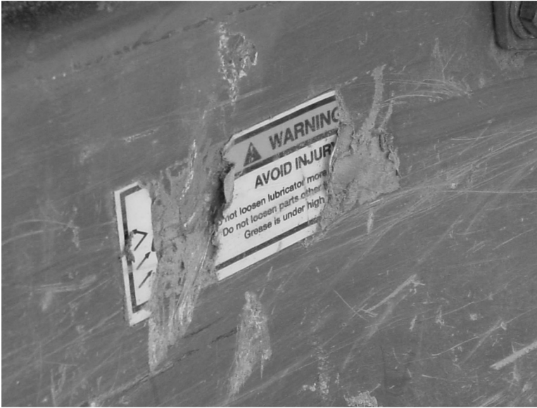
FIGURE 9.9A Warning label rendered useless by abrasion. Labels must be designed, manufactured, and placed to withstand the expected conditions of use for the product.
