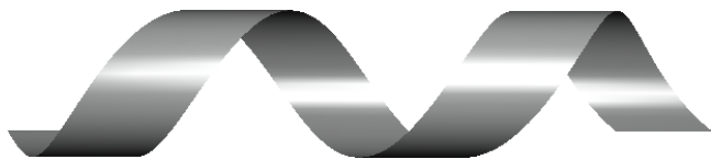
Figure 7.8: Ruled surface of the tangents to a cylindrical helix.
