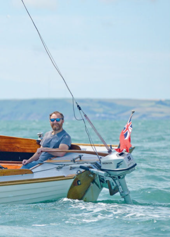
A pronounced sheer, high bow and clinker strakes help the boat handle waves
