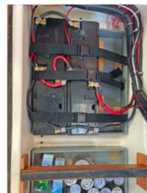
Bank of LFP lithium batteries gives more usable capacity
