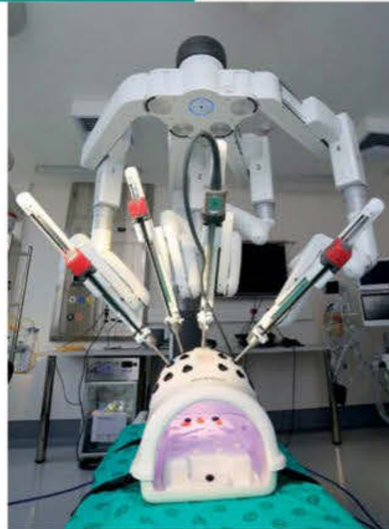
The components of the Da Vinci Xi Robot as they would be arranged in a theatre.
